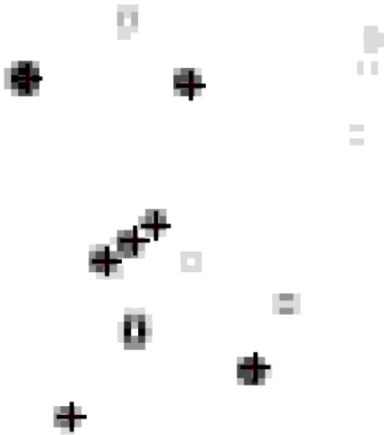
Figure 10. Star mapping of Orion constellation onto CCD chip. In this roughly 30 x 30 pixel region, "+" shows the anticipated locations based on lens calibration, and gray boxes show star images.
