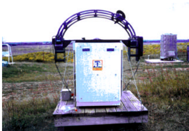
Figure 1. Day/night whole sky imager fielded at SGP CART site. (For a color version of this figure, please see http://www.arm.gov/docs/documents/technical/conf_9803/shields-98.pdf .)
